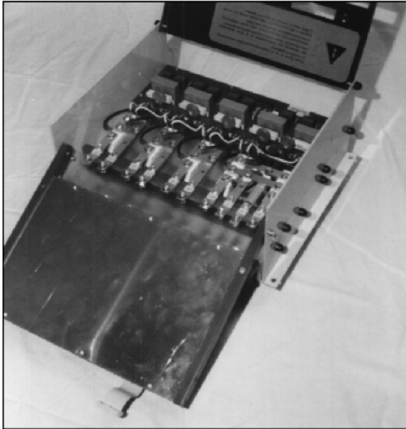
Figure 3.7 Swinging up the front panel, swinging down the printed board (in the picture you can see the rear aluminium shielding plate; the released ribbon connector for the power section is visible at the bottom).
